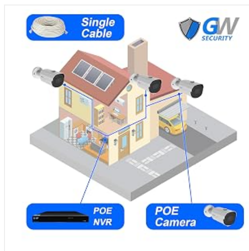
Figure 4.1: Diagram illustrating Power over Ethernet (PoE) connection from NVR to camera.
