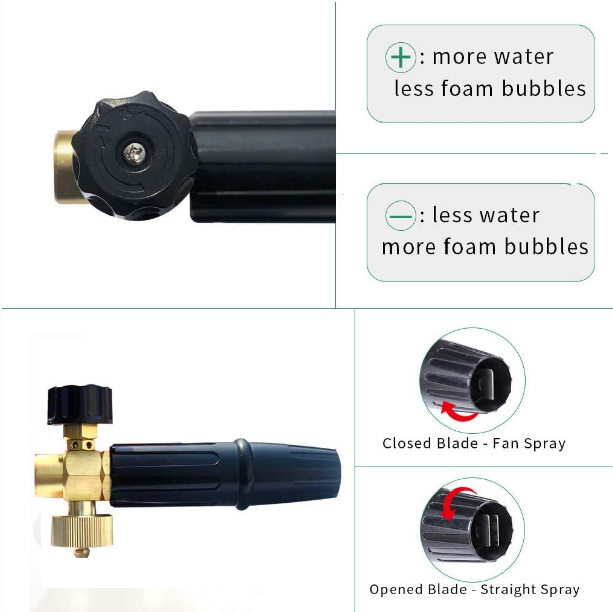
Figure 4: Adjusting foam concentration and spray pattern.
