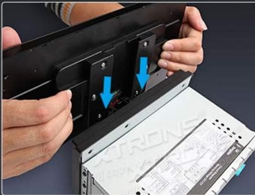
**3** Make the face panel back side get through the head units' holder from top, then lose hold of the face panel.
