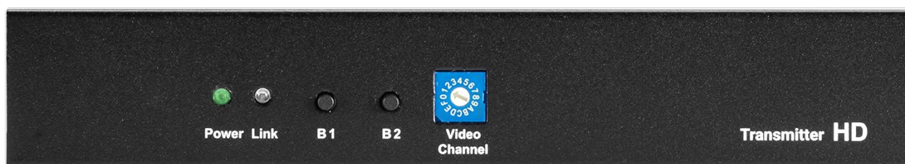
Figure 1: Front panel view of the MediaCento IPX HD Extender Transmitter. This view shows the Power, Link, B1, B2 indicators, and the Video Channel selector dial.
