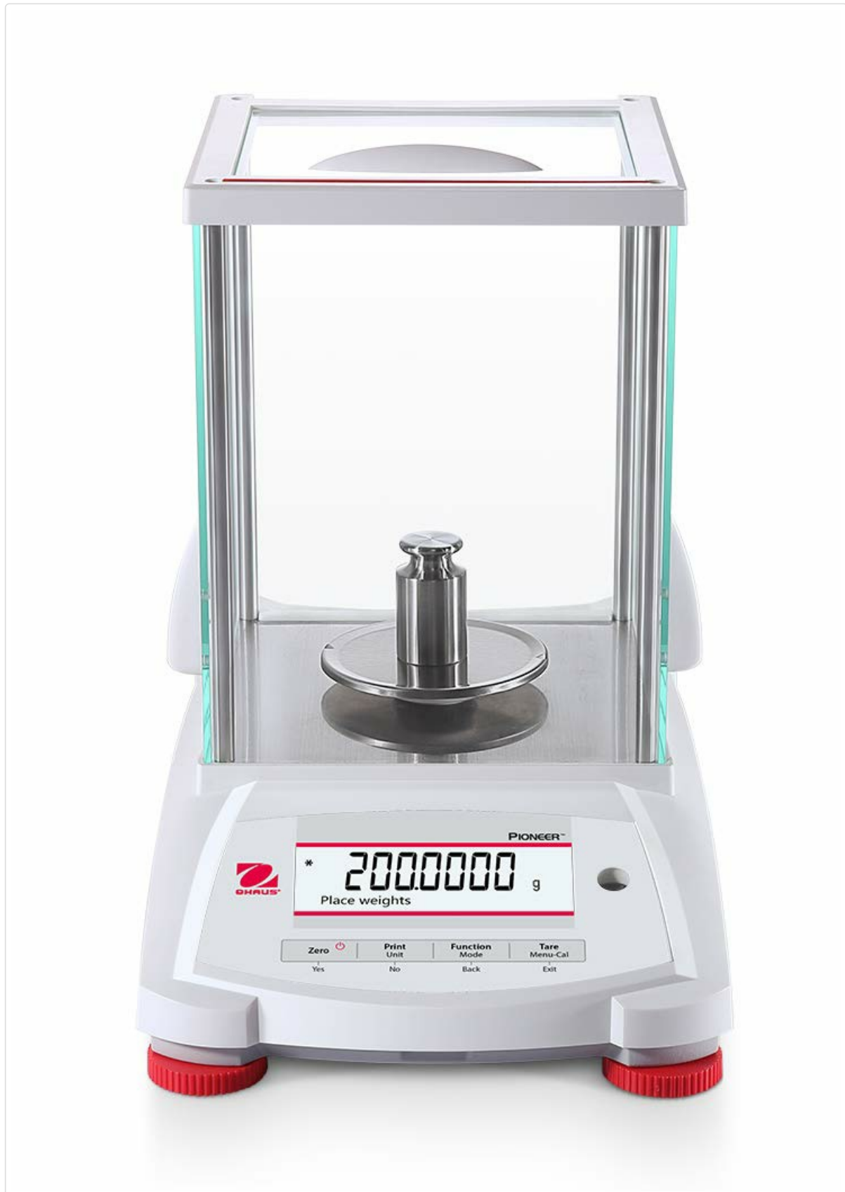
Figure 5.1: The balance displaying a stable weight reading with a calibration weight placed on the weighing pan.
