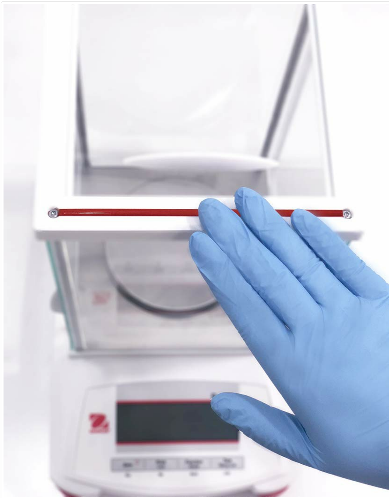
Figure 5.2: A hand demonstrating the use of the static removal bar to dissipate static electricity.
