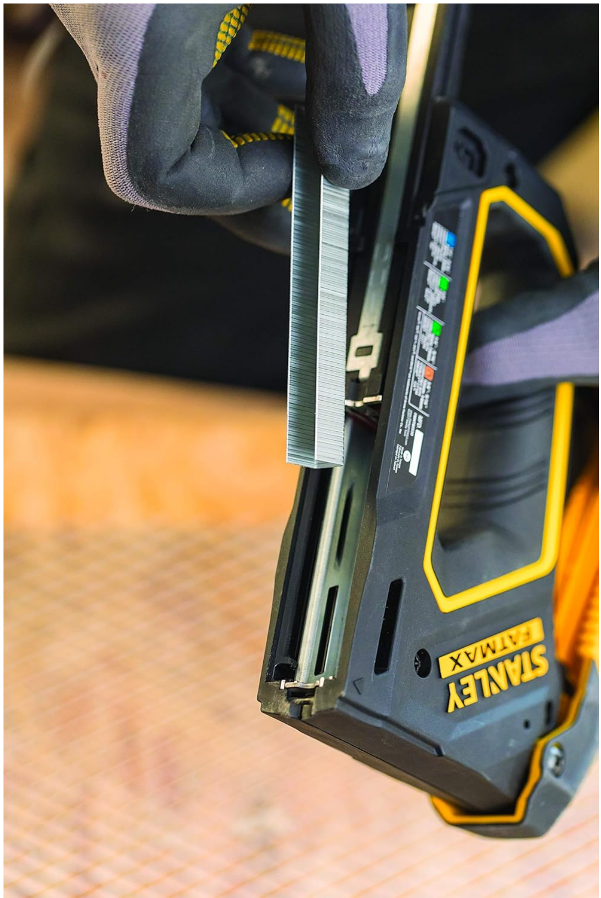
Image 4.1: Demonstrating the rear-loading process for staples into the magazine.
