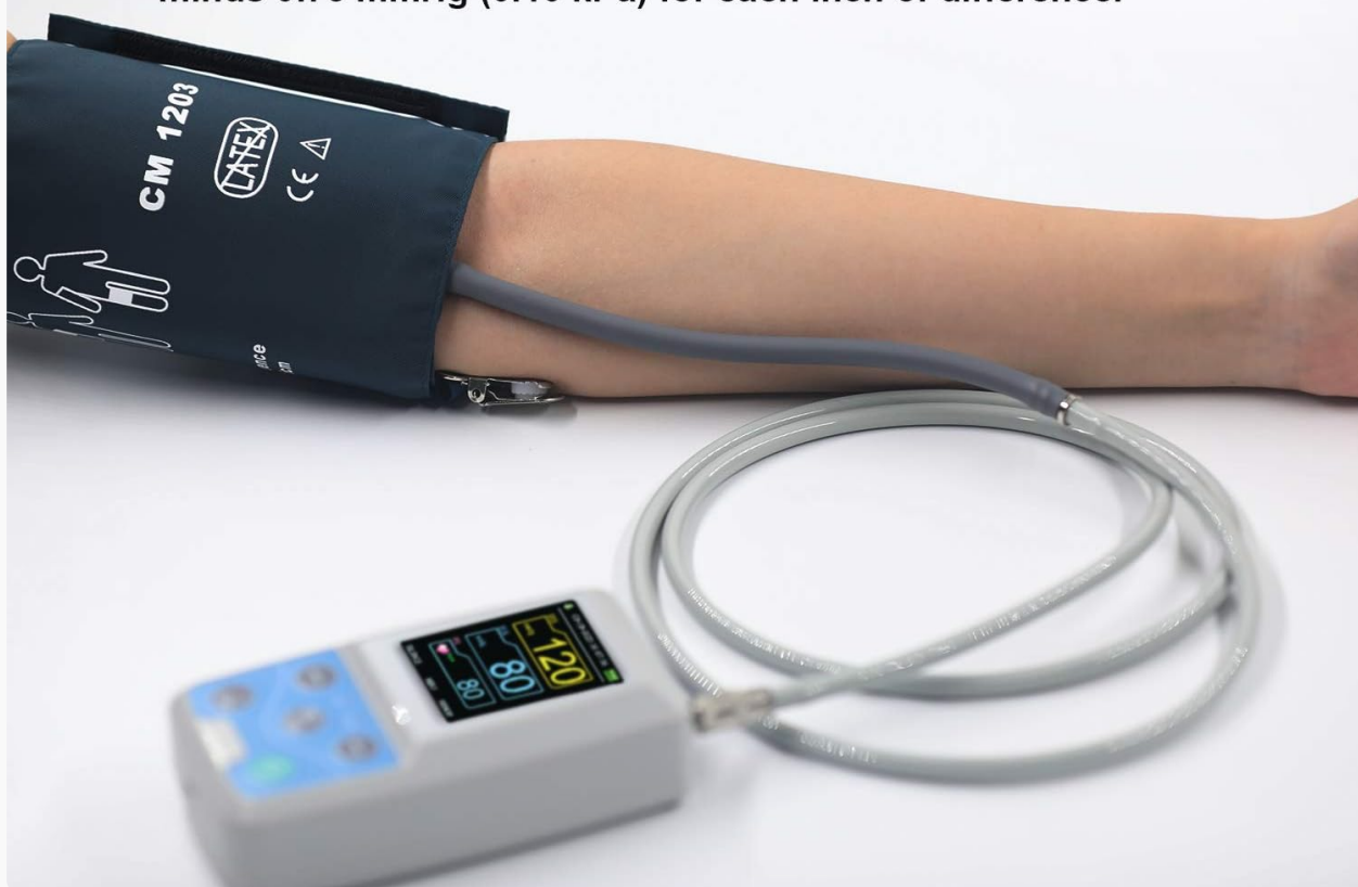
Figure 4.1: Illustration of proper cuff placement on the upper arm, with the monitor unit connected via the extending tube. The cuff should be at the same level as the patient's heart for accurate readings.
