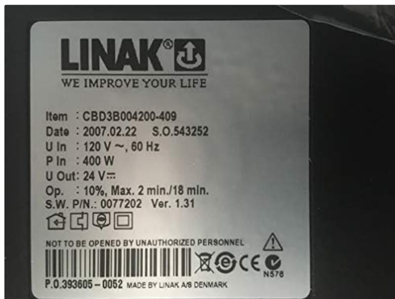
Figure 2: Close-up of the product label on the LINAK CBD3 Control Box. The label displays critical information such as item number (CBD3B004200-409), date of manufacture, input voltage (120 V~, 60 Hz), power input (400 W), output voltage (24 V---), operation cycle (10%, max. 2 min./18 min.), and software P/N. It also includes safety certifications and a barcode.
