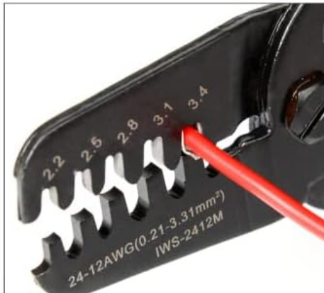
Figure 5.1: Step-by-step visual guidance for using the crimping tool, illustrating how to place a parallel barrel into the upper die and insert a stripped wire into the barrel. A diagram shows the conductor and insulation barrels.
