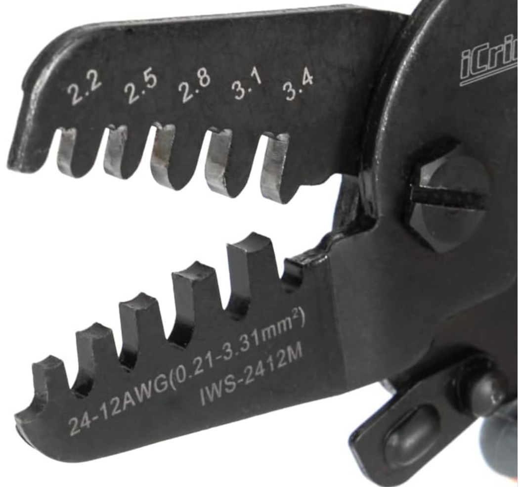
Figure 2.2: A detailed view of the crimper's polished jaws, highlighting the five die widths (2.2mm, 2.5mm, 2.8mm, 3.1mm, 3.4mm) and the AWG 24-12 (0.21-3.31mm 2 ) capacity markings.
