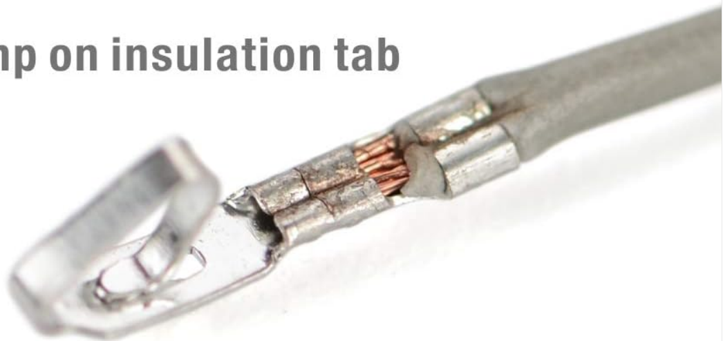
Figure 5.2: Close-up images demonstrating correctly crimped terminals, showing both the conductor tab crimp and the insulation tab crimp.
