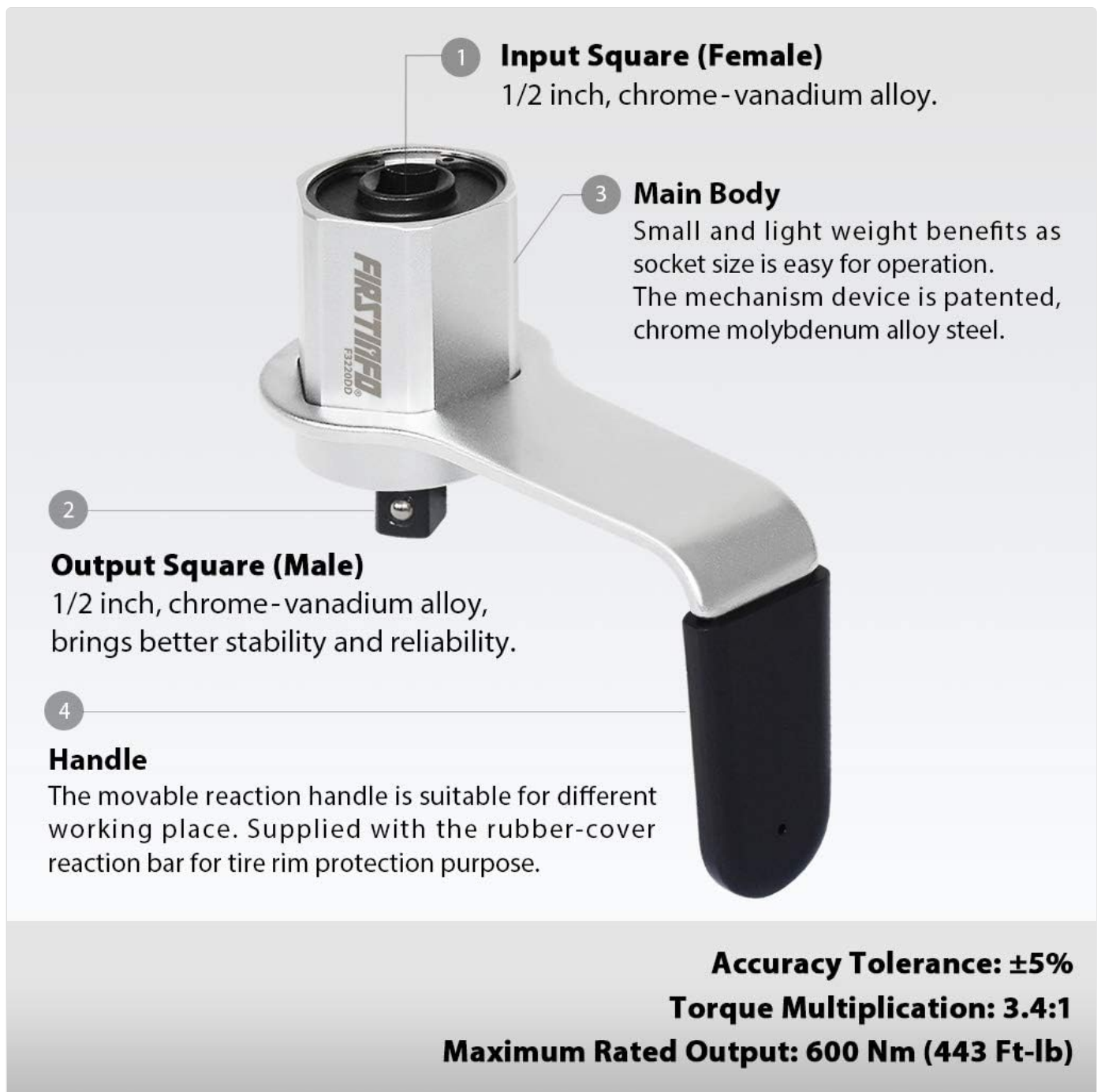
Figure 2.1: Key components of the F3220DD Torque Multiplier.
