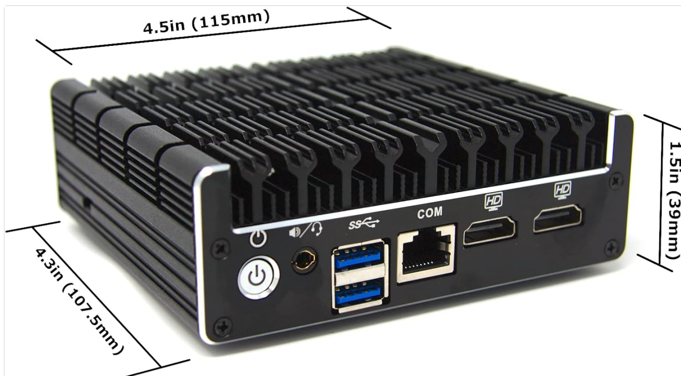
Figure 4: Rear panel of the FW2B, including the power button, audio jack, two USB 3.0 ports, one RJ-45 COM port, and two HDMI ports.
