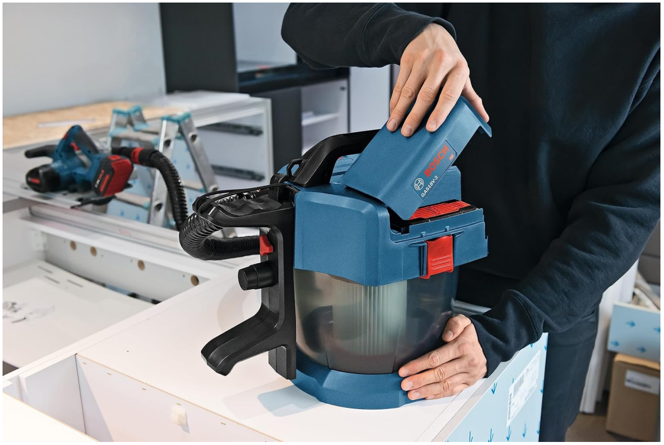
Figure 4.1: Proper insertion of an 18V battery into the vacuum's battery compartment.
