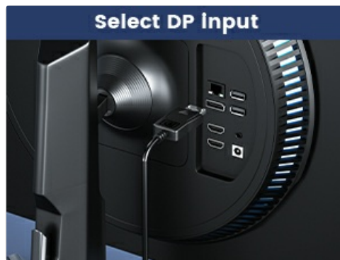
Figure 3: Connecting the DisplayPort cable from the adapter to your display.
