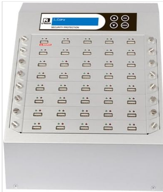
Figure 1: Front view of the U-Reach UB940S USB Duplicator. This image shows the device's front panel, including the LCD screen, control buttons, and 40 USB ports arranged in rows. The screen currently displays '1. Copy', indicating a copy operation is selected.
