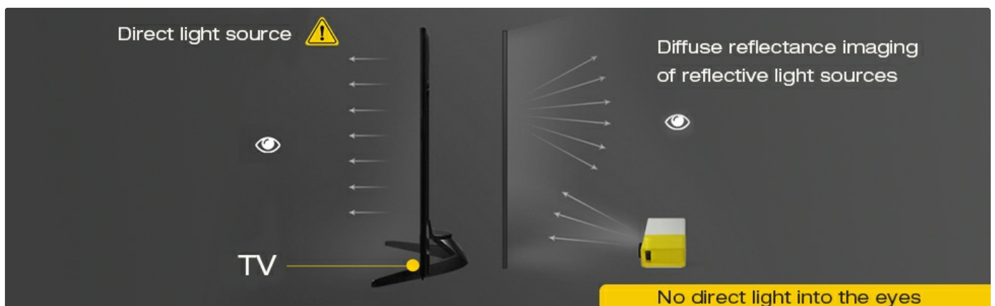
Image: Explanation of diffuse reflectance imaging, which prevents direct light from entering the eyes, making it safer for viewing.
