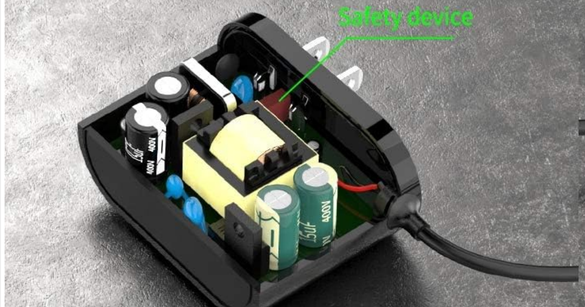
Image: A close-up view of the adapter's internal components and its fireproof PC enclosure, highlighting the robust construction and safety features.
