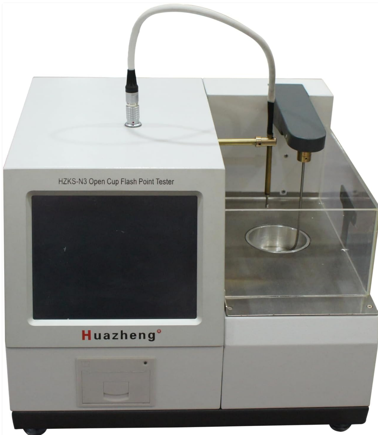
Figure 1: HZKS-3 Open Cup Flash Point Tester. This image shows the main unit with its integrated screen on the left and the open cup testing area on the right, including the igniter arm and temperature probe.
