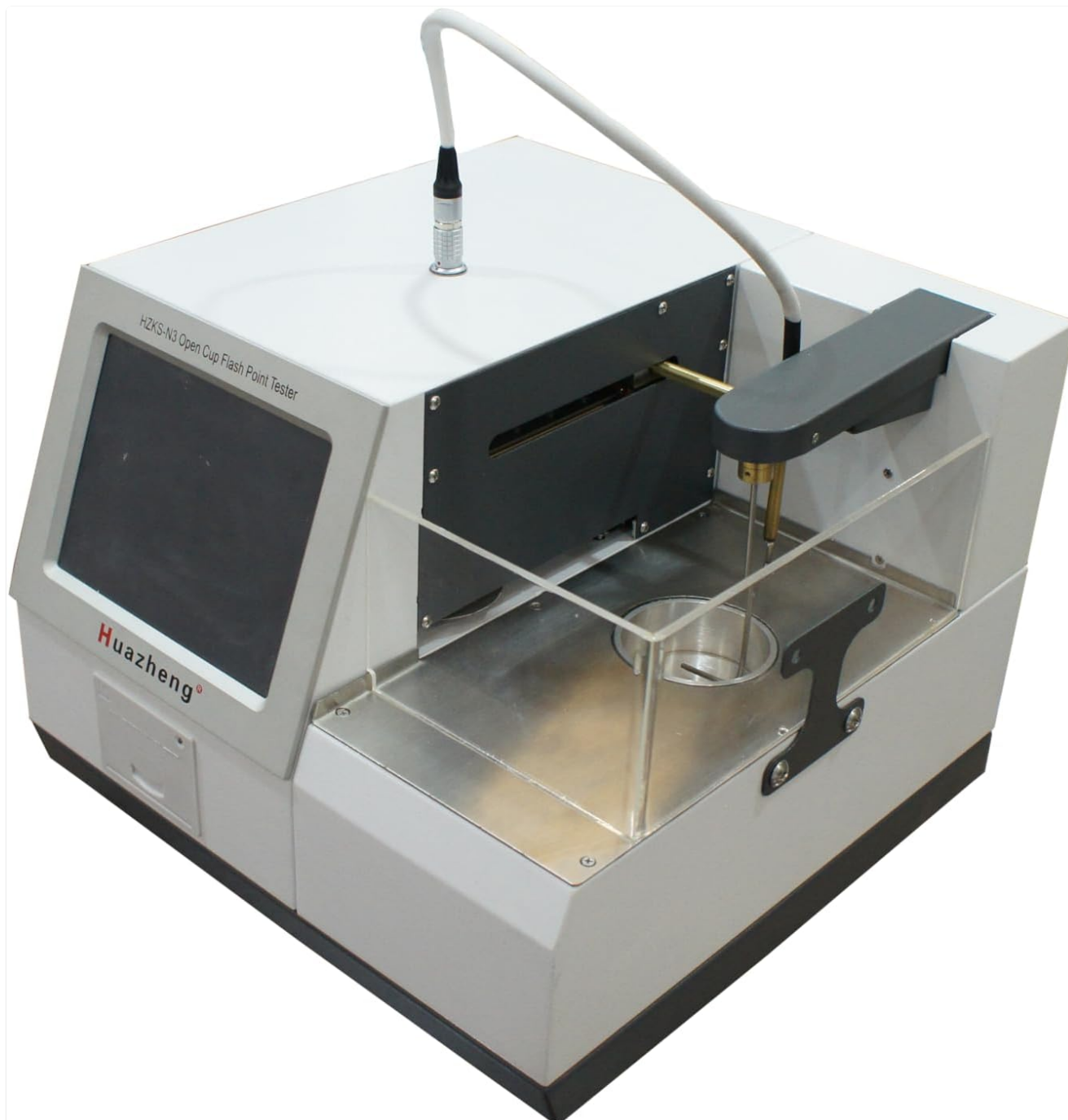
Figure 3: Angled view of the HZKS-3 tester. This image provides a clearer view of the instrument's overall design, including the screen interface and the open cup area with its protective cover.
