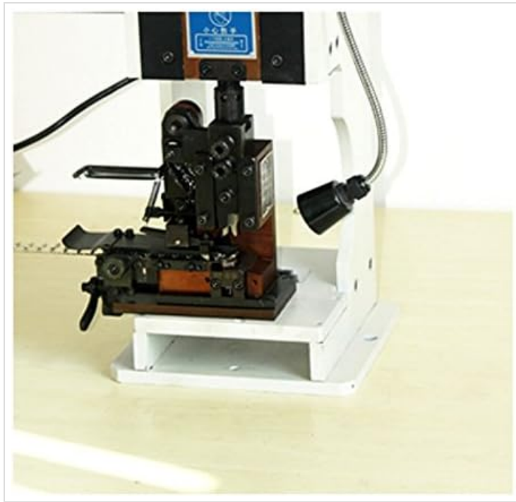
Figure 4: Detailed view of the crimping mechanism, showing the area where terminals and wires are inserted.
