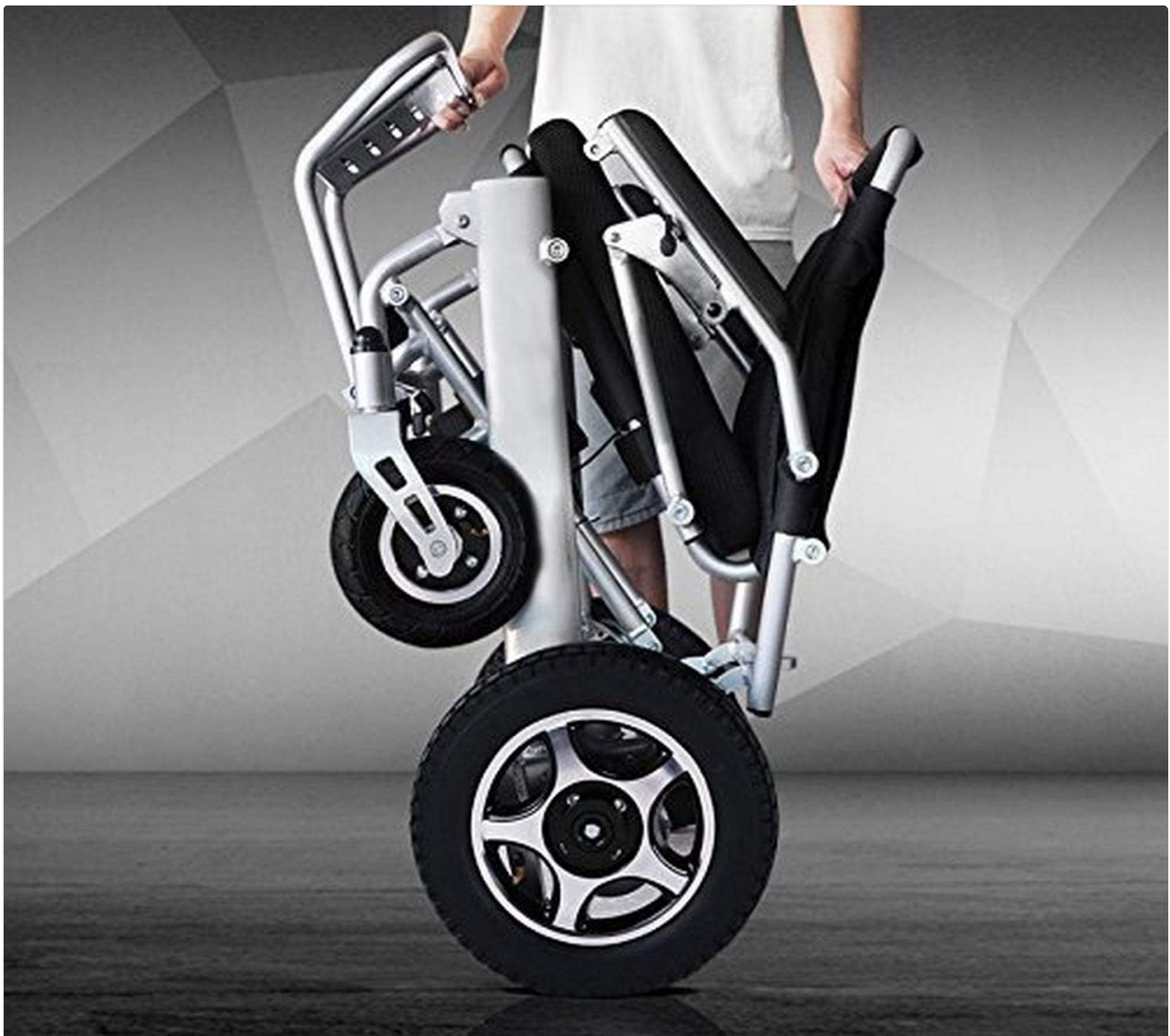
Figure 3.2: Folding for Transport
