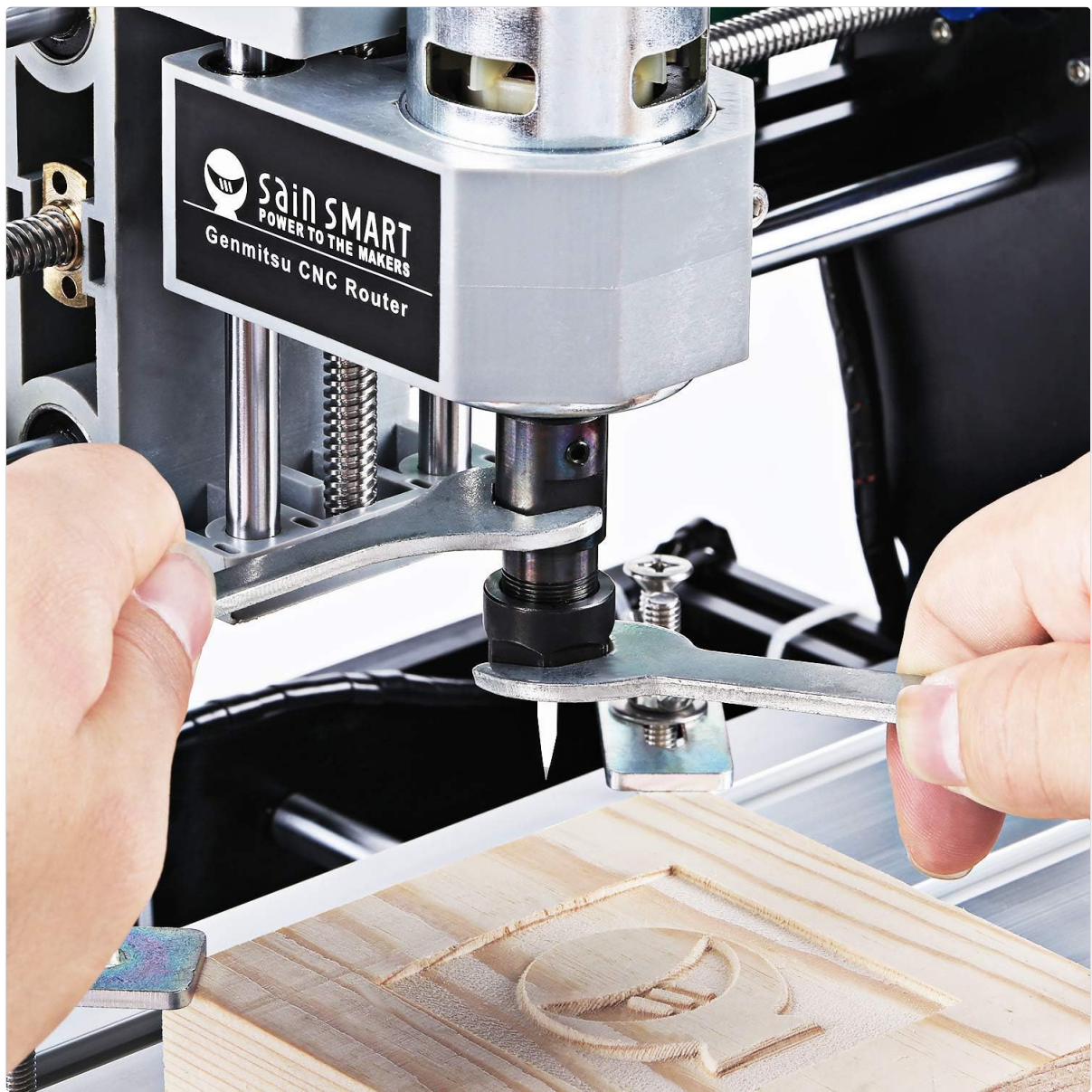
Figure 5.3: Proper method for securing a milling bit into the ER11 collet using the provided wrenches.
