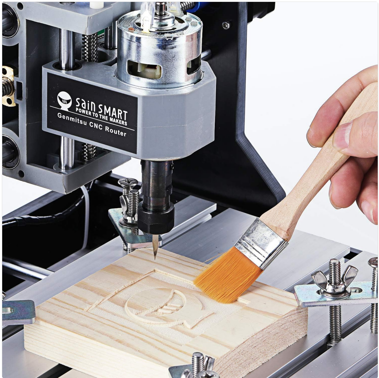
Figure 5.4: Clearing debris from the workpiece and machine bed after a milling operation.
