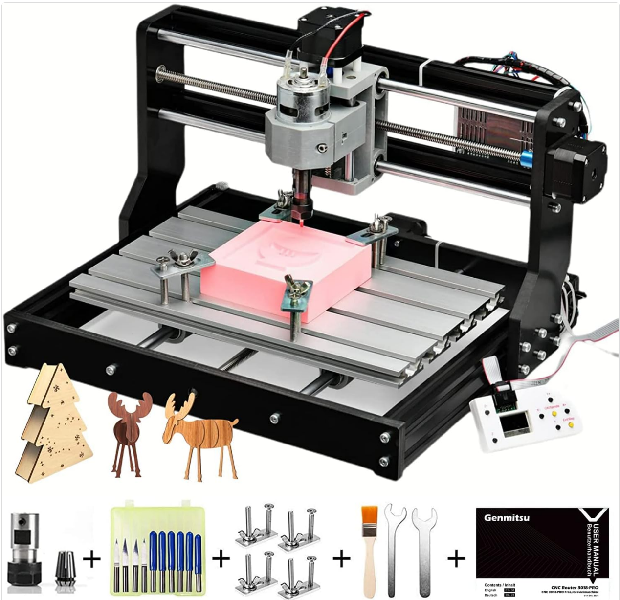
Figure 3.2: The assembled Genmitsu 3018-PRO CNC machine, showcasing its compact design and included accessories like clamps and bits.
