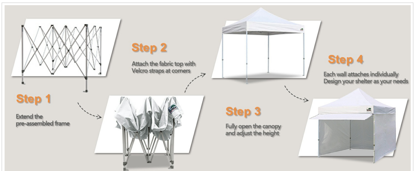
Figure 2: Extend the pre-assembled frame.
