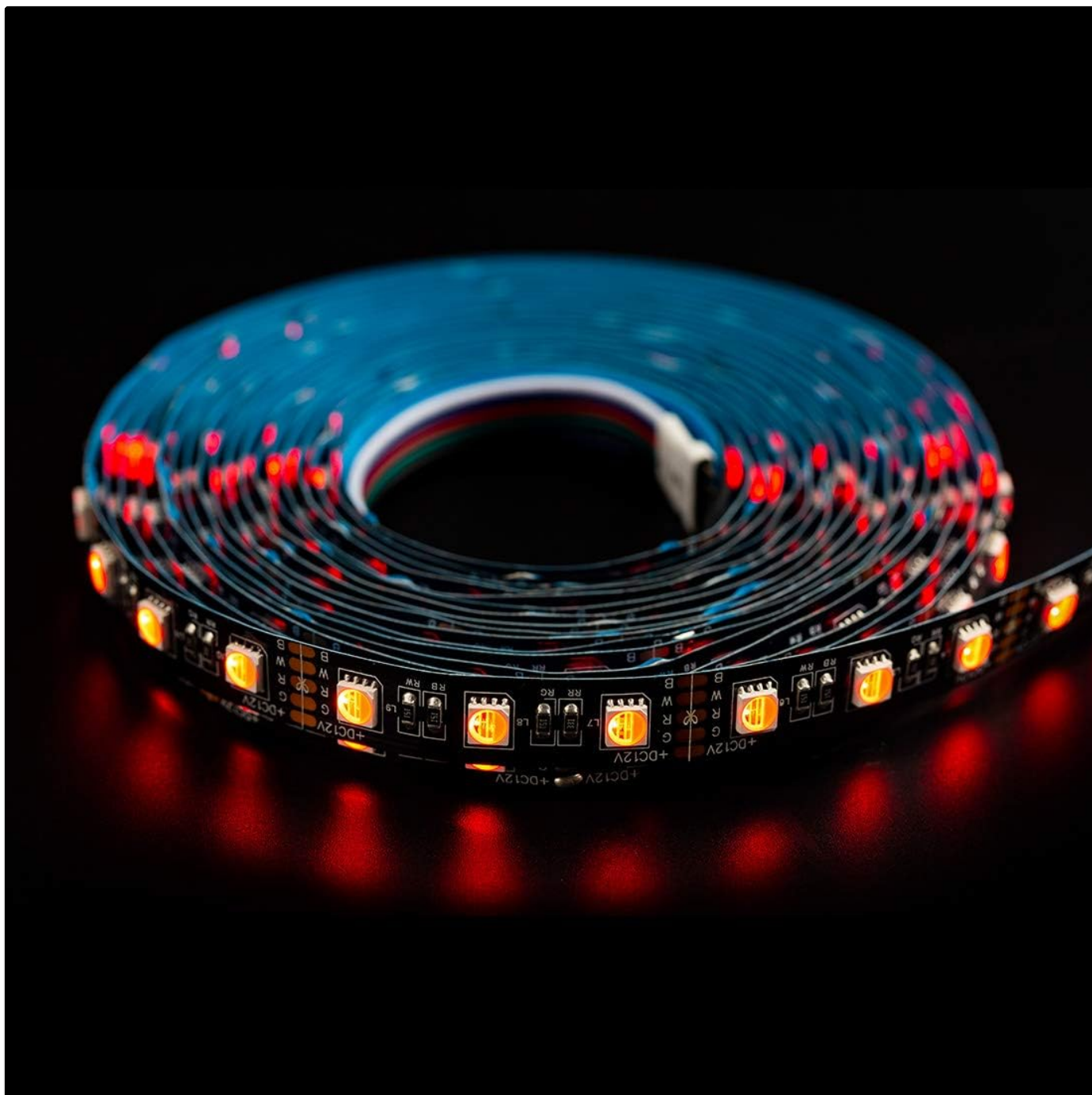
Image: A detailed view of the LED strip, highlighting the connection points and the segments where it can be safely cut.
