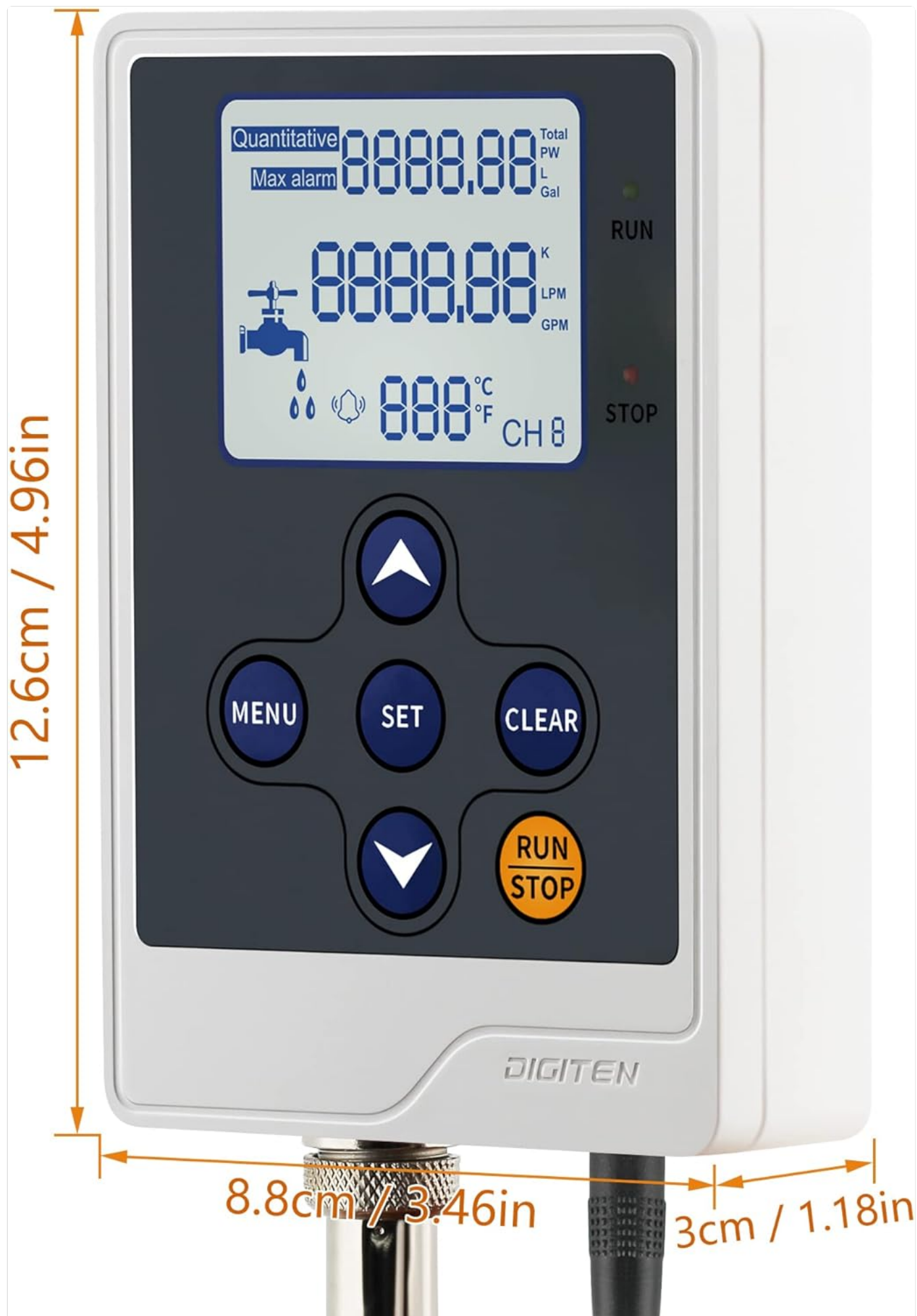
Figure 6.1: Front panel of the DFC15 controller showing the LCD display and control buttons (MENU, SET, CLEAR, UP, DOWN,
