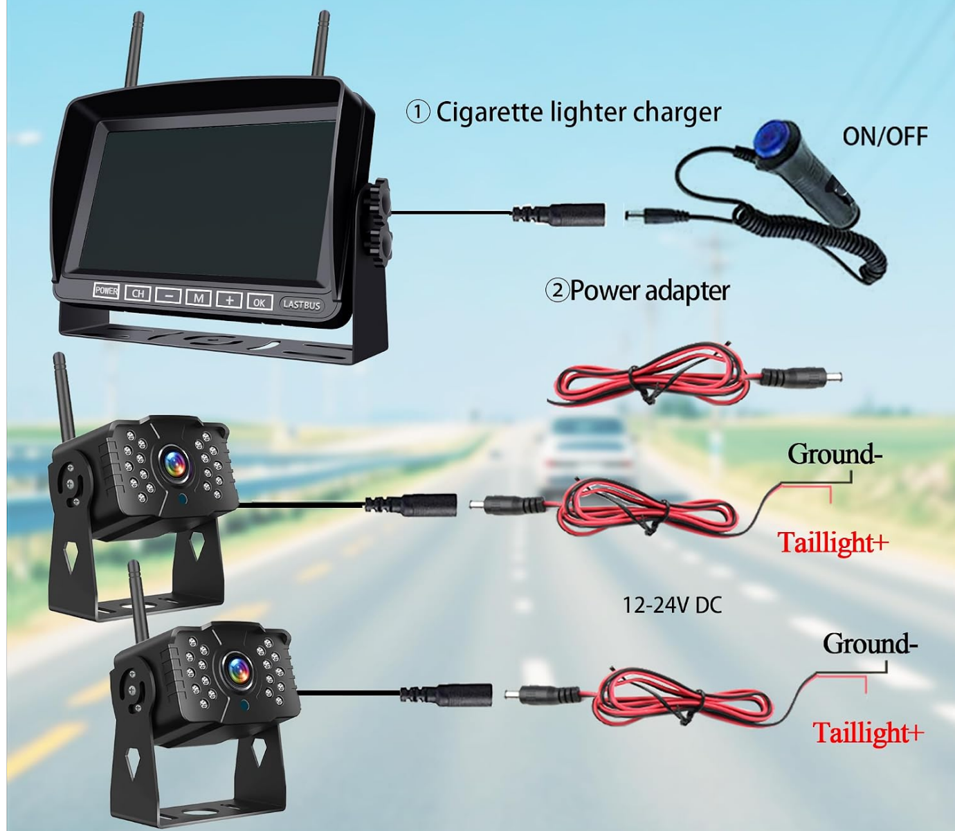
Image: Installation diagram illustrating power connections for the monitor and cameras.
