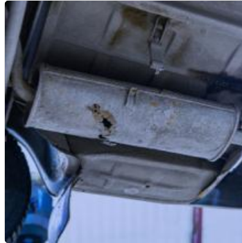
Figure 7: An image showing a rusted muffler under a vehicle, indicating a common reason for replacement.
