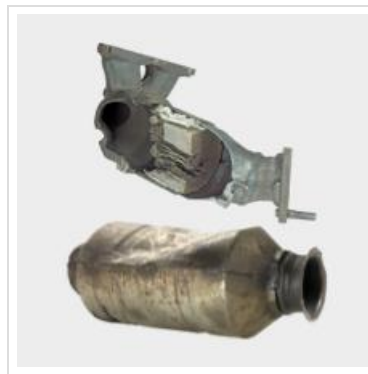
Image: A cutaway view of a catalytic converter, revealing the internal honeycomb structure coated with catalytic materials responsible for emissions conversion.
