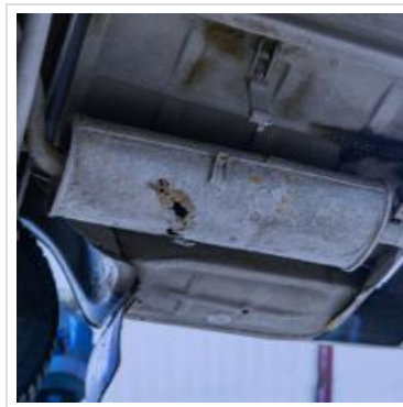
Image: A view of a rusted and damaged muffler assembly under a vehicle, indicating the need for replacement.
