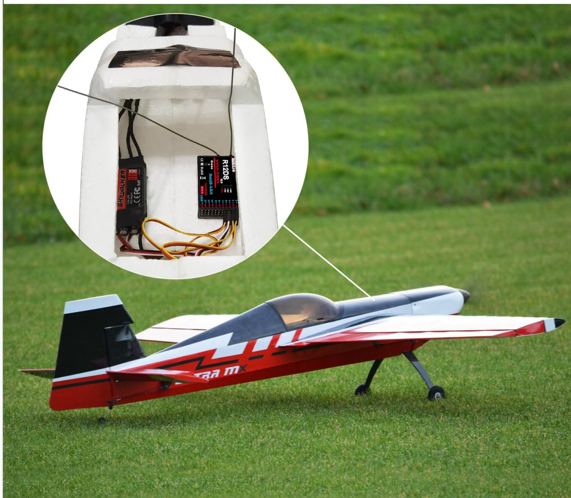
Image: Compatible Radiolink Transmitters. This image illustrates the R12DS receiver's compatibility with AT9/AT9S/AT9S Pro and AT10/AT10II transmitters.
