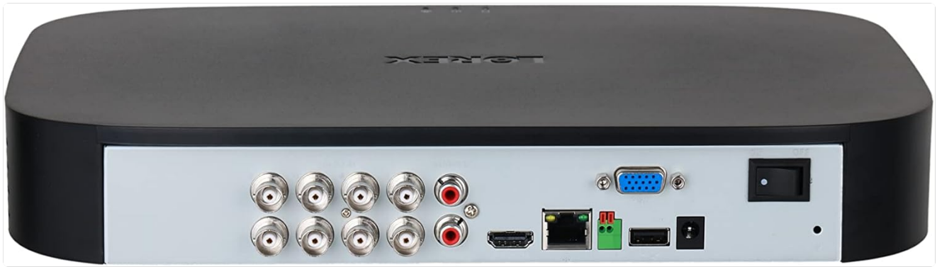
Image 2.1: Rear panel of the DVR with connection ports.
