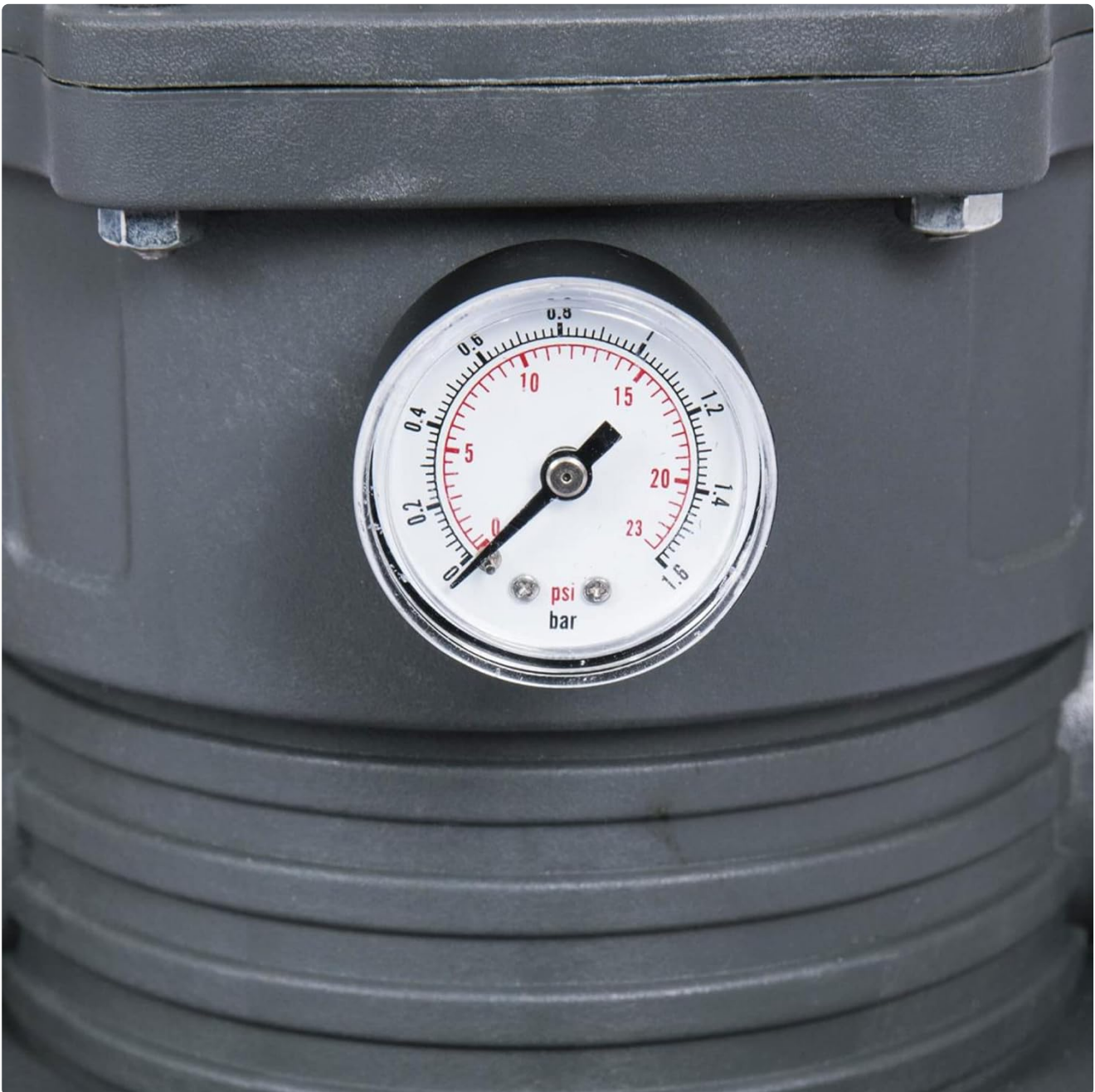
Figure 5: Pressure gauge indicating the operating pressure of the filter system.
