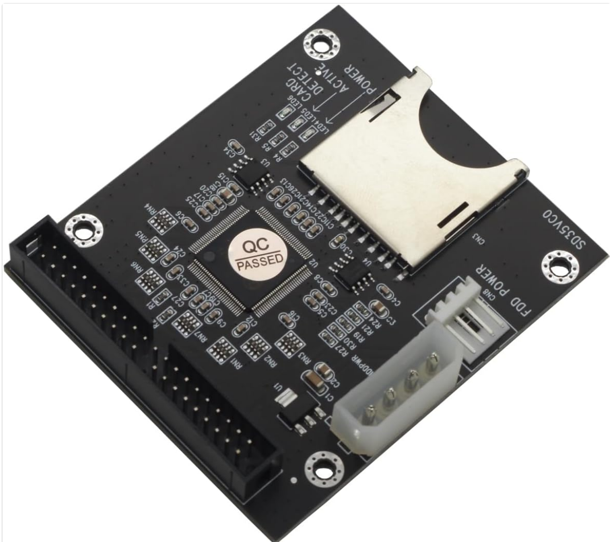
Figure 2: Close-up of the 40-pin male IDE connector for motherboard connection.
