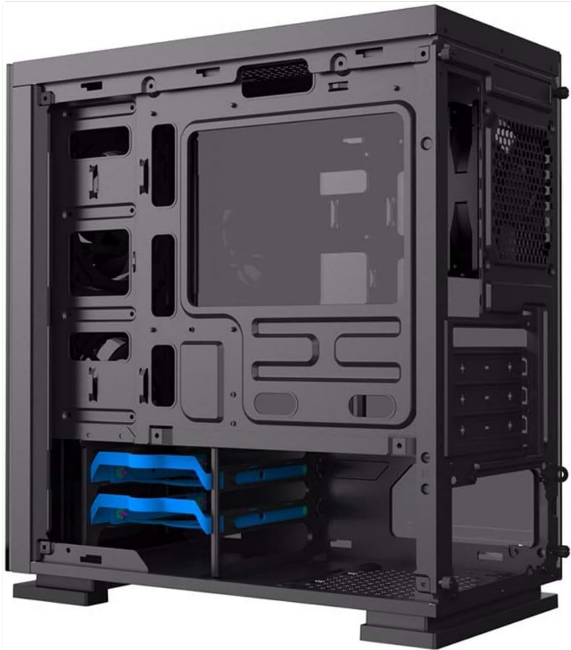
Figure 4: View of the internal 3.5-inch HDD drive bays (blue trays).
