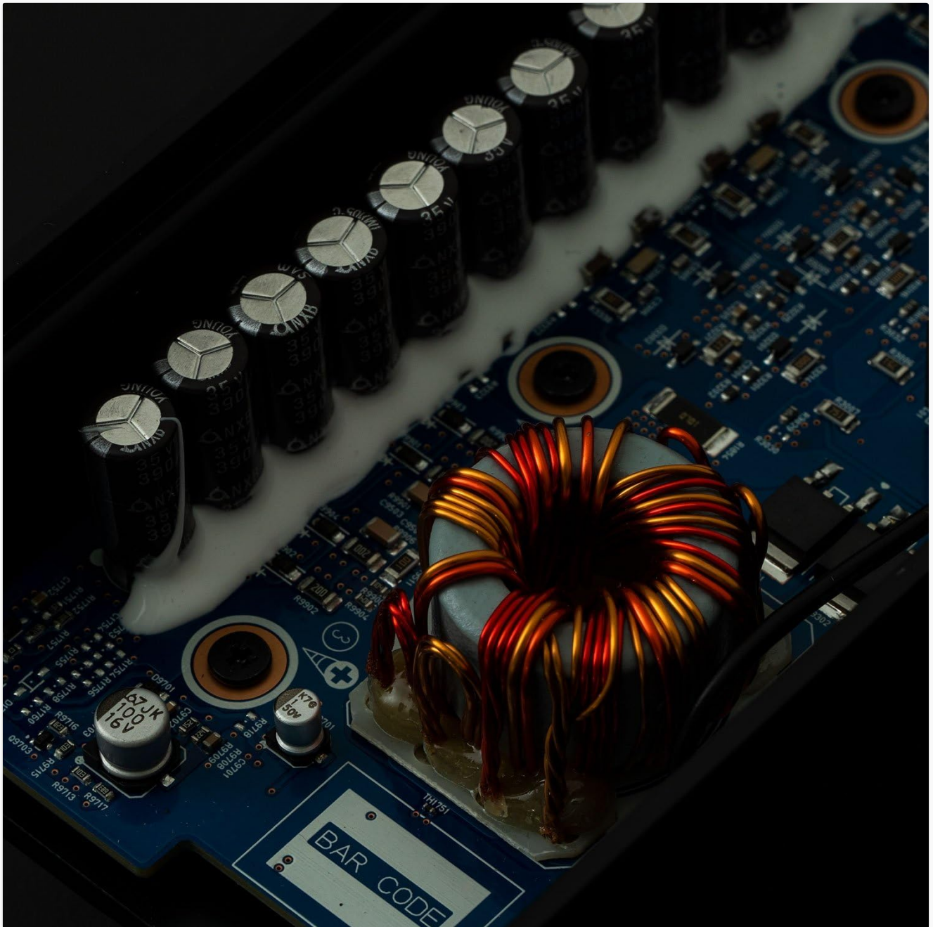
Image 2: Internal view of the Alpine KTP-600 circuit board, highlighting the digital components responsible for sound processing and power delivery.
