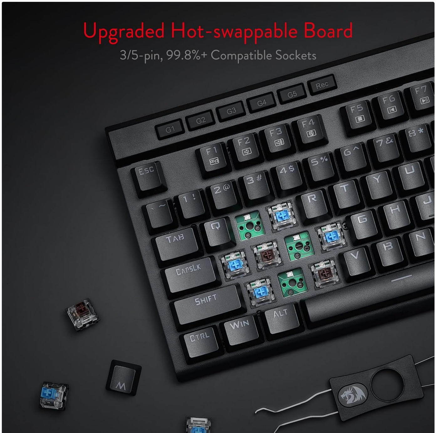
Figure 6: Hot-swappable switch sockets on the Redragon K580.
