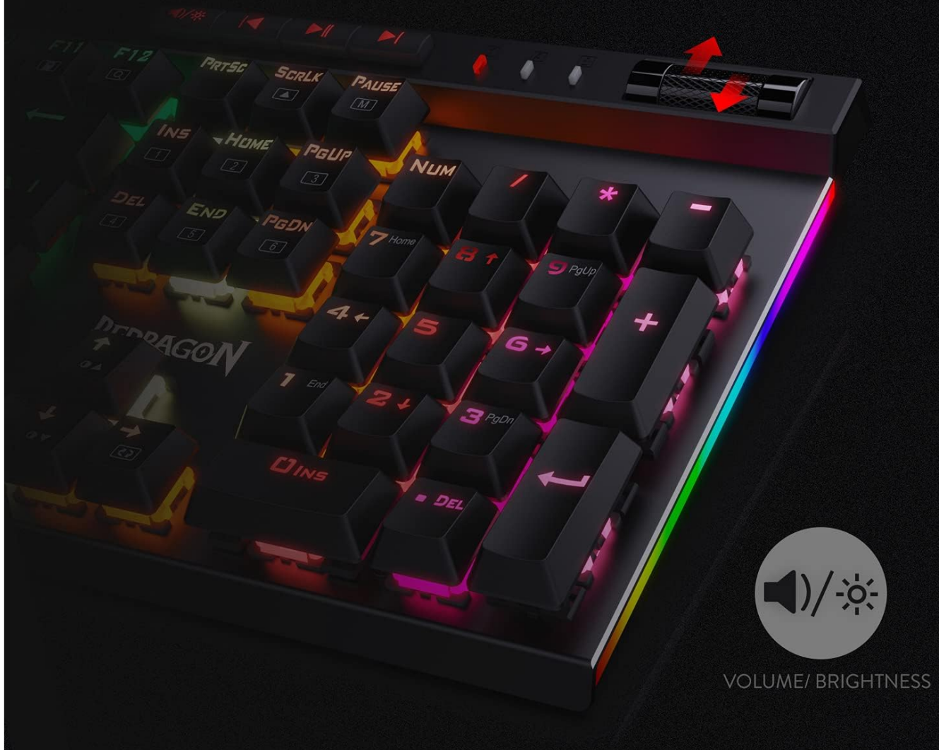
Figure 4: Multi-function scroll bar for volume and backlight brightness control.
