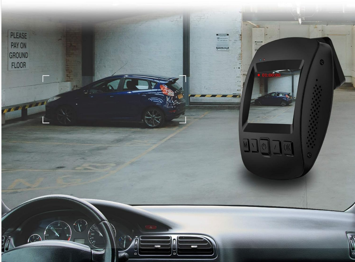
Image: Illustration of the G-Sensor function, which automatically locks video files during a collision to secure accident evidence.
