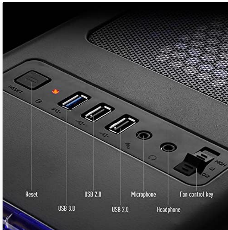
Figure 3.2: Top I/O Panel layout.
