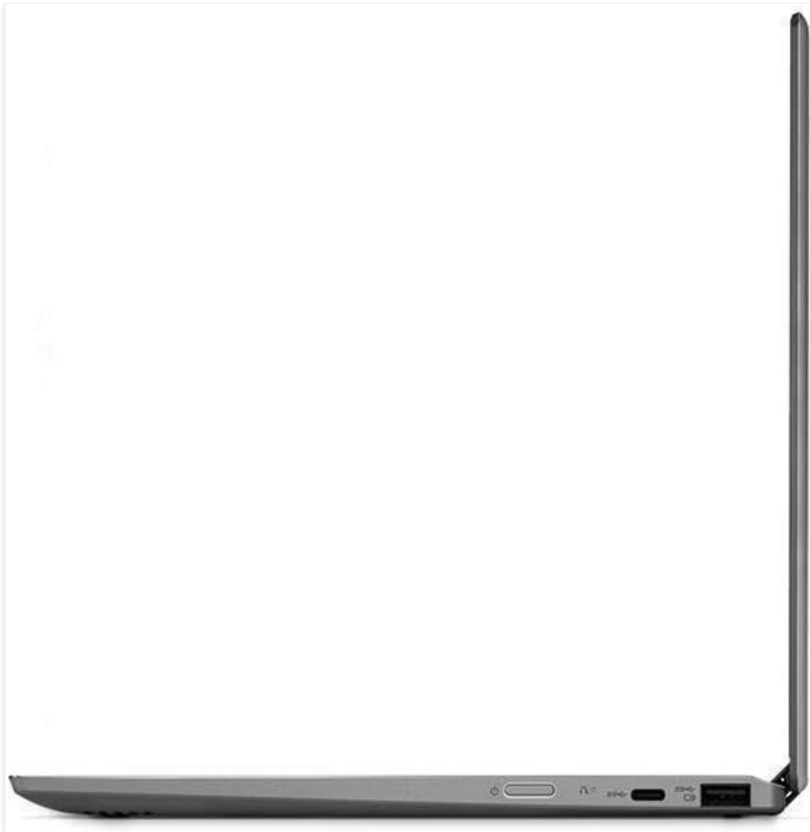
Figure 3: Right side view of the device, featuring a USB-C Thunderbolt port, a USB 3.0 port, and the power button.
