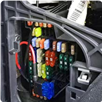
Image: A diagram illustrating the correct placement of the original car fuse and the dash cam fuse into a fuse tap.
