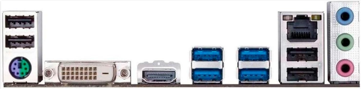
Image 5.1: Rear I/O panel, showing HDMI, DVI-D, USB, LAN, and audio ports for connecting external devices.
