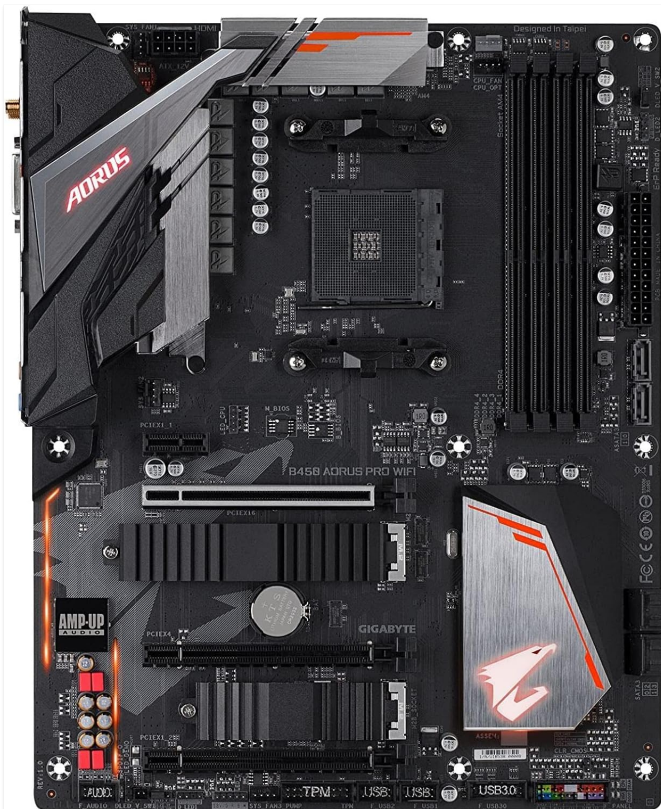
Figure 2.1: Top-down view of the motherboard, highlighting key component locations such as the CPU socket, DIMM slots, and M.2 slots.
