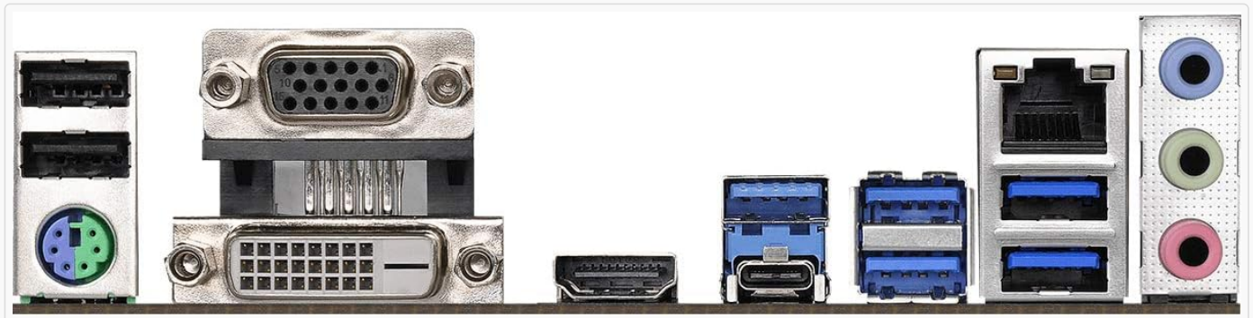
Image: Close-up view of the rear I/O panel of the ASRock B450M PRO4 motherboard, showing various ports including USB, HDMI, DVI, VGA, and audio jacks.
