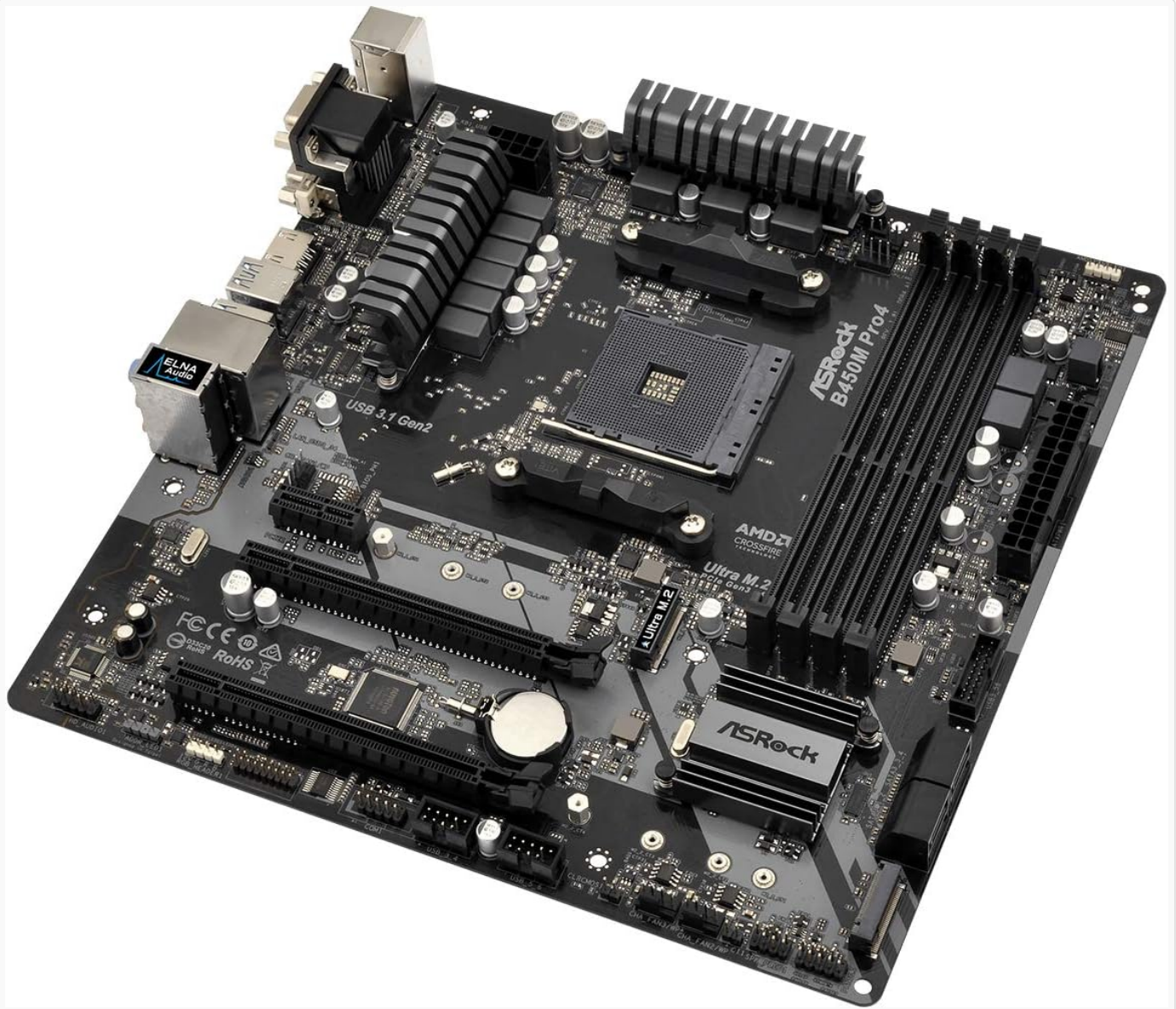
Image: Angled view of the ASRock B450M PRO4 motherboard, providing a clearer perspective of the heatsinks and various connectors.
