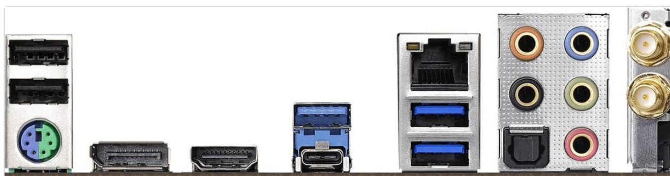
Figure 5: Detailed view of the ASRock B450 Gaming-ITX/AC Motherboard's rear I/O ports, including USB, LAN, audio, and Wi-Fi antenna connectors.
