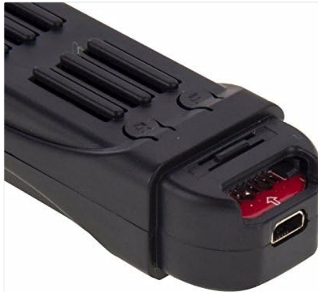
Figure 4: A detailed close-up of the T189 Mini DV Camera's Mini USB port and the Micro SD card slot, showing the internal components.
