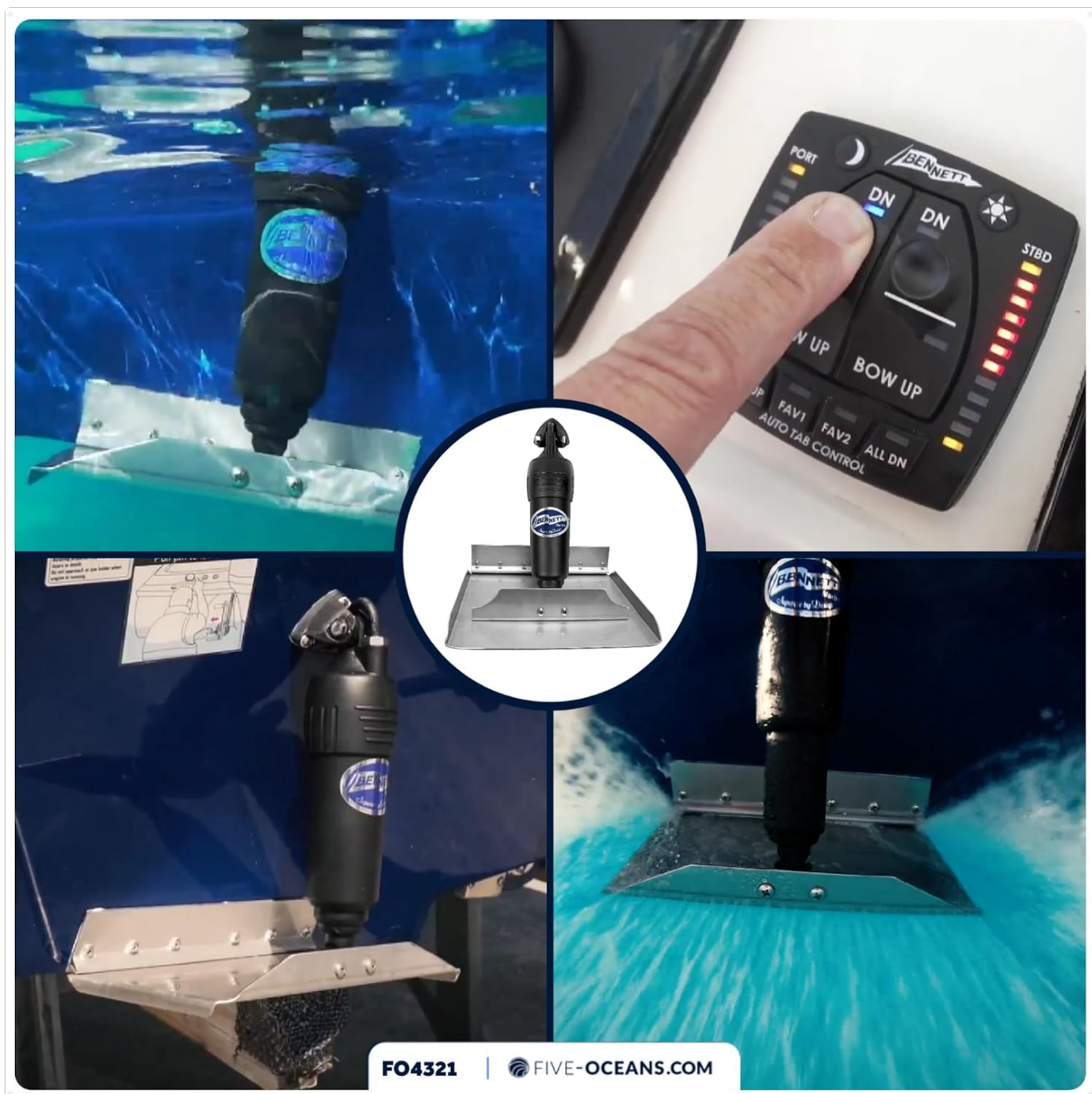
Figure 8: Various views of the trim tabs and helm control in action, demonstrating how the system adjusts the boat's running attitude.
