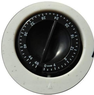
D. Time setting eg. it will open after around 2.3 hrs
