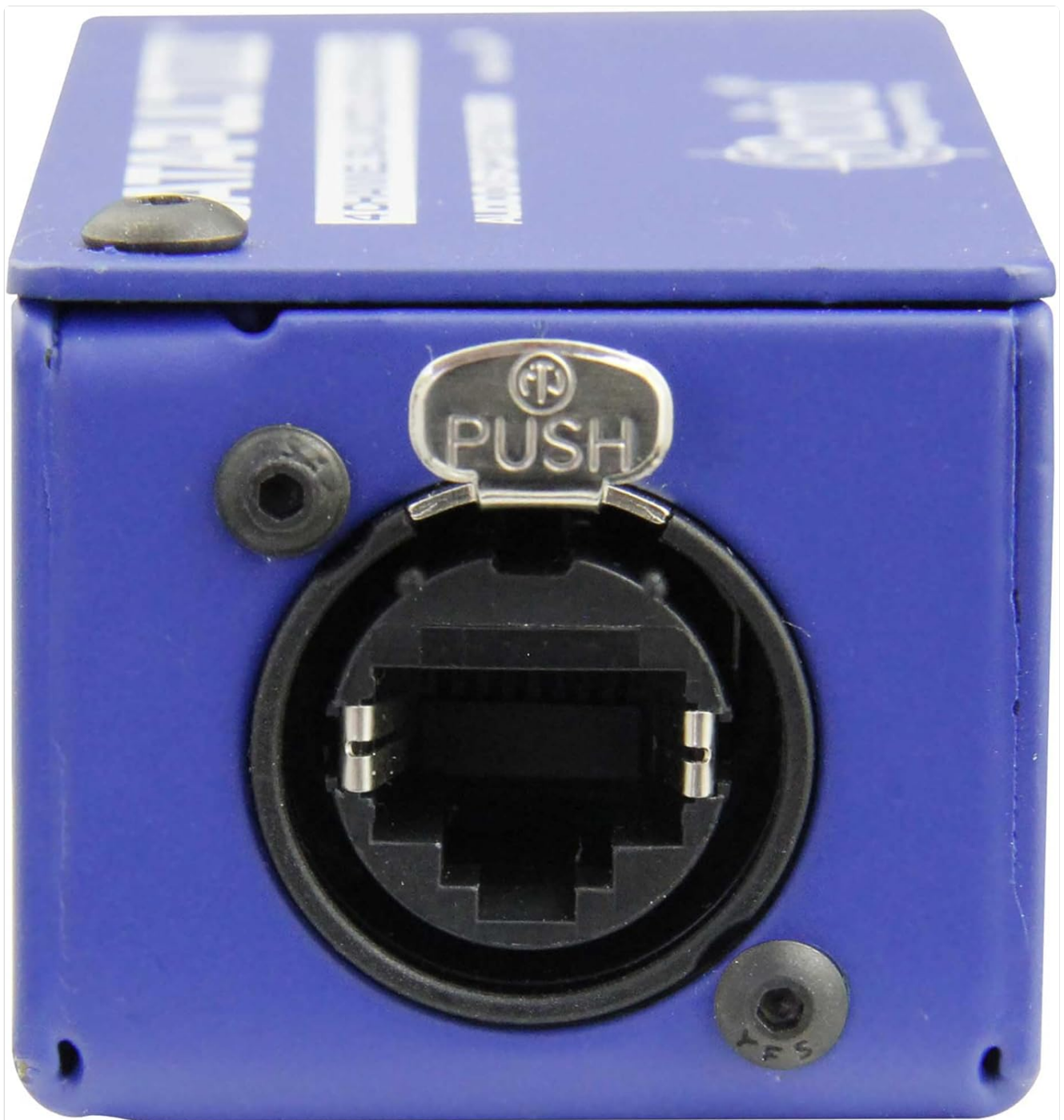
Figure 3: End view of the Catapult MINI TX, highlighting the RJ45 and XLR connector ports.
