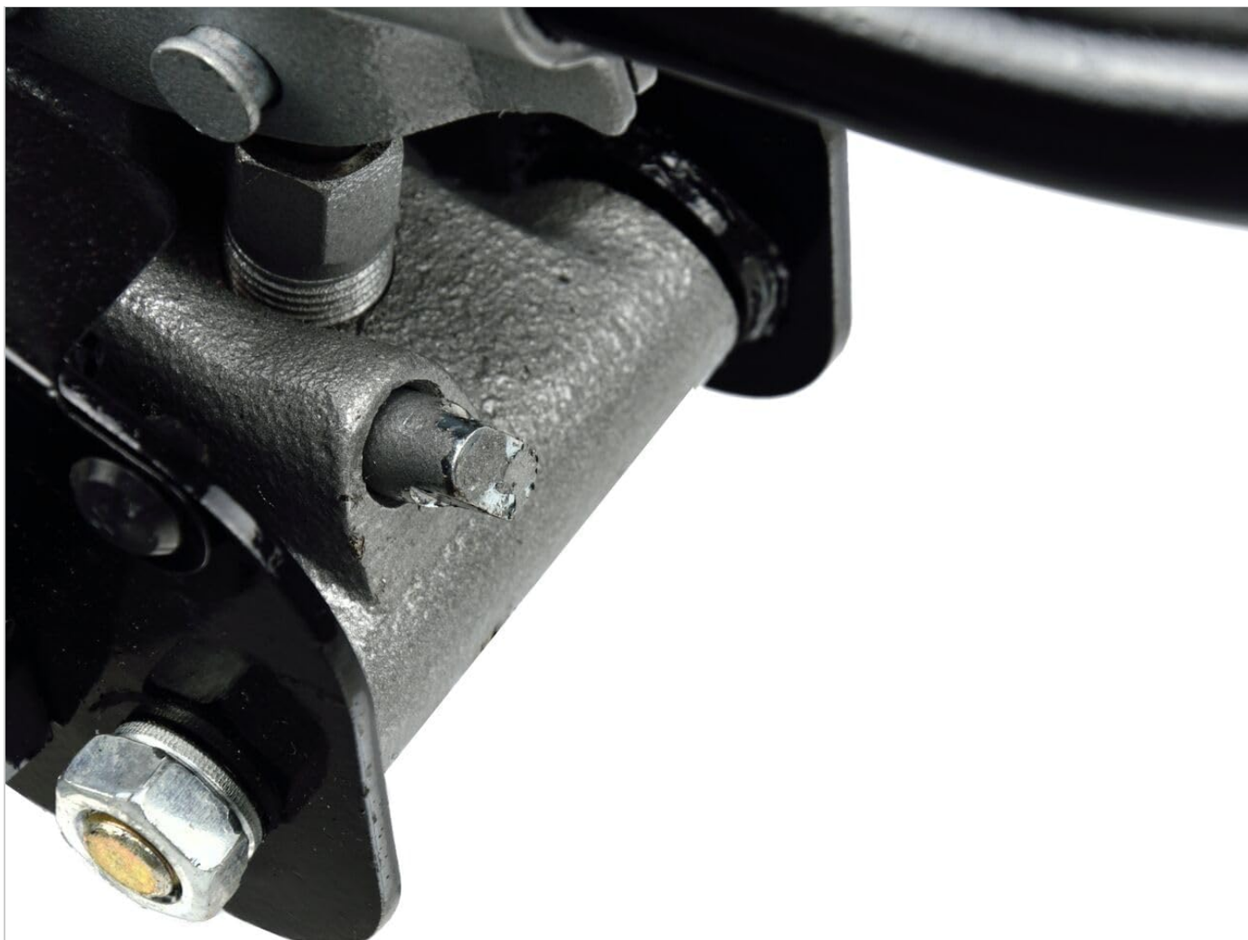
Image 3.8: A detailed view of the hydraulic release valve mechanism on the Geko G02032 jack. This component is crucial for controlling the lowering speed of the jack.
