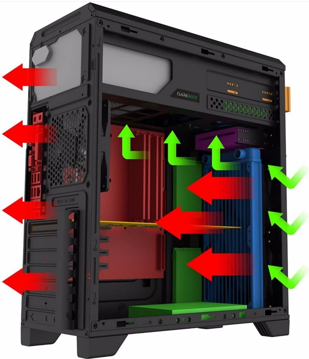
Image 2.1: Diagram illustrating the recommended airflow within the GAMEMAX G561 case, showing intake and exhaust paths.
