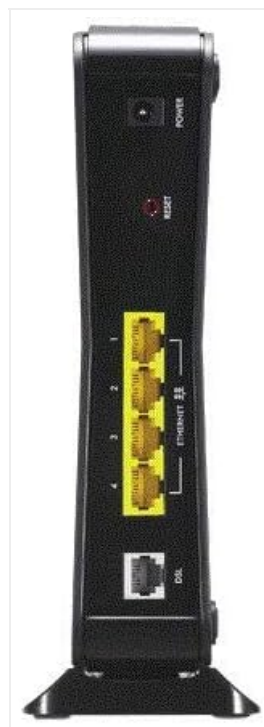
Figure 3: Rear view of the ZYXEL P660HN-51R showing ports and connections.
