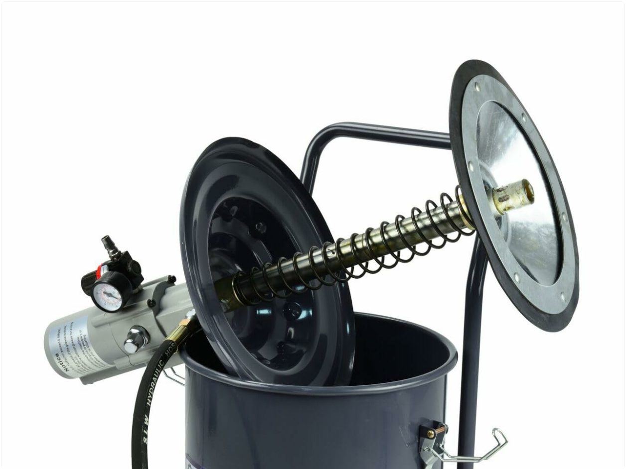
Figure 4: View inside the grease container, showing the follower plate and spring mechanism designed to push grease towards the pump inlet.
